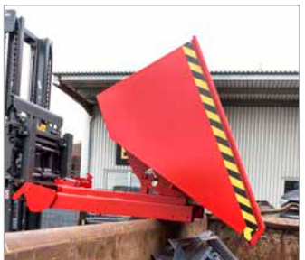
Emptied by activating release point 2
