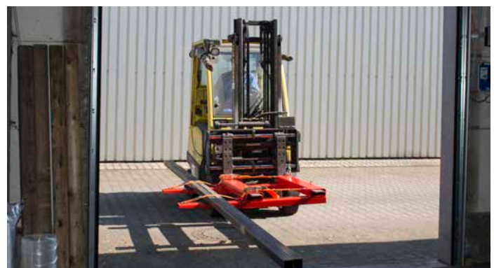
Use the LSL for long material and easily pass through gates or navigate narrow aisles
