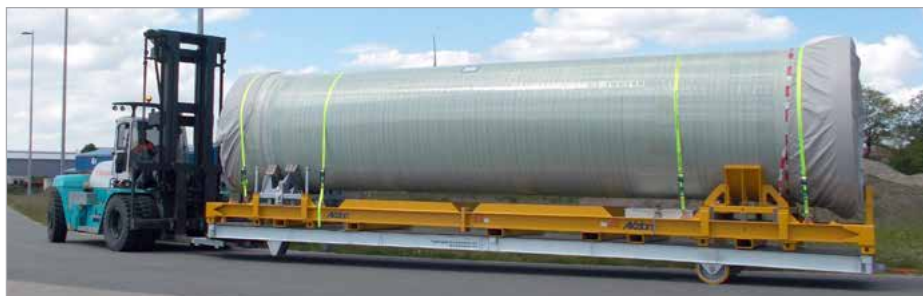
Used to transport extremely heavy and bulky components; 12 m long, load capacity 20 t
