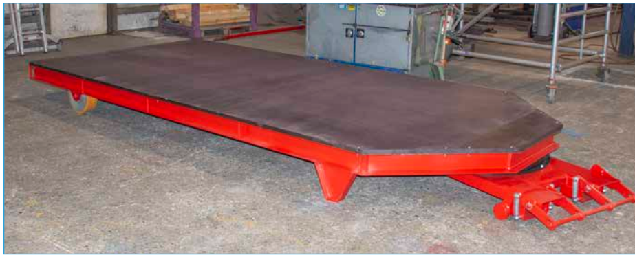
STS with anti-slip "Betosieb" boards
