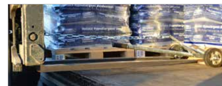
Drawing the pallet into the "front row" using a forklift truck
