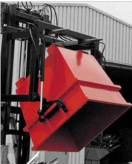
UC and Hydraulic Traverse Type UCT
