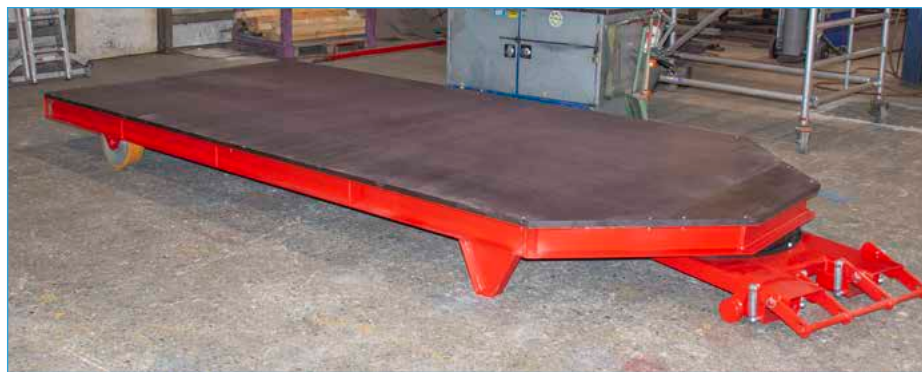
STS with anti-slip "Betosieb" boards
