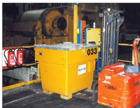
Mobile oil supply for machines
