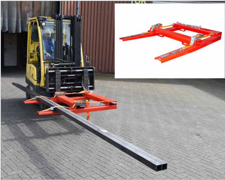
Pick-up position for transport, for example through gates or passages
