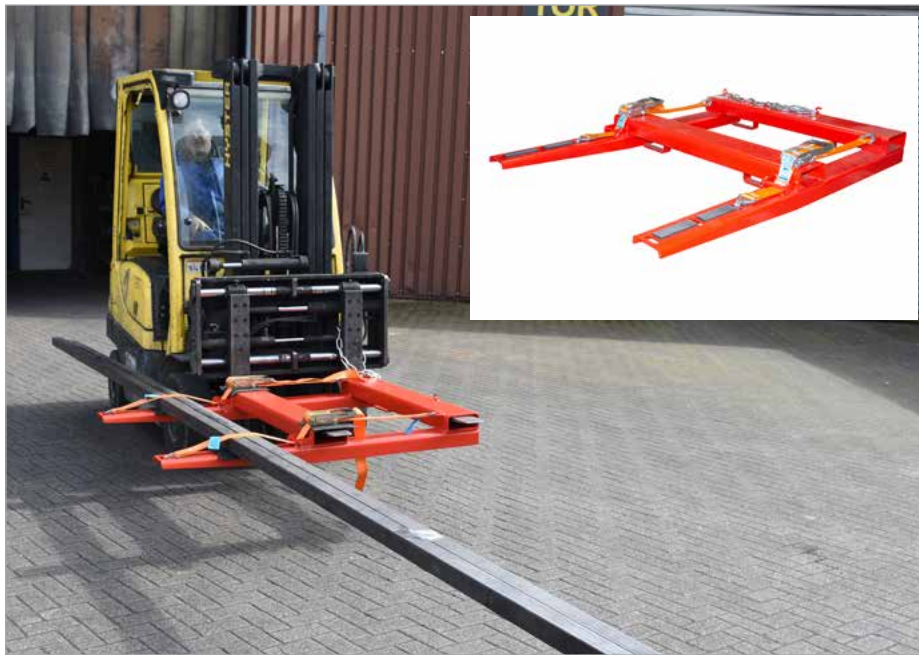
Pick-up position for transport, for example through gates or passages
