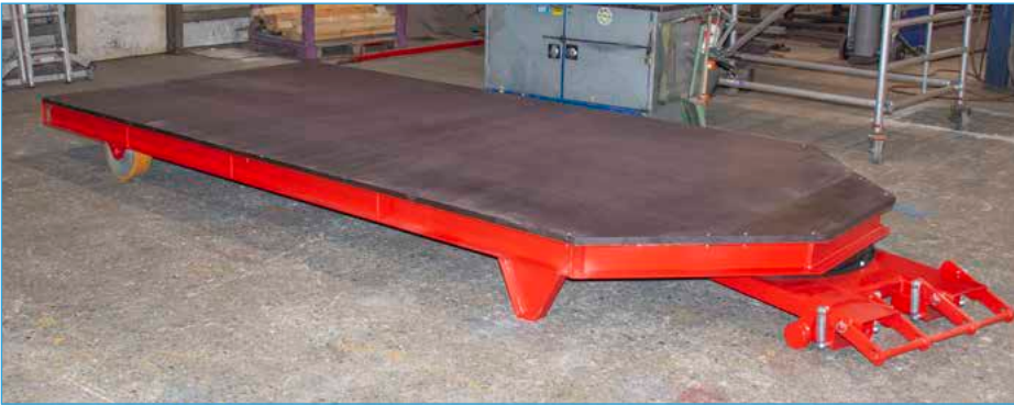
STS with anti-slip "Betosieb" boards
