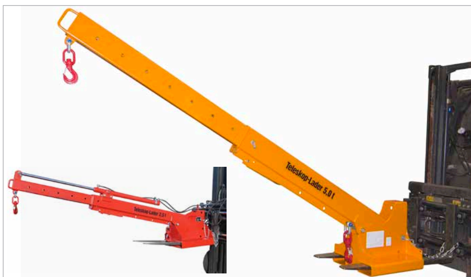
Hydraulic extension function (KTH) (accessories)
