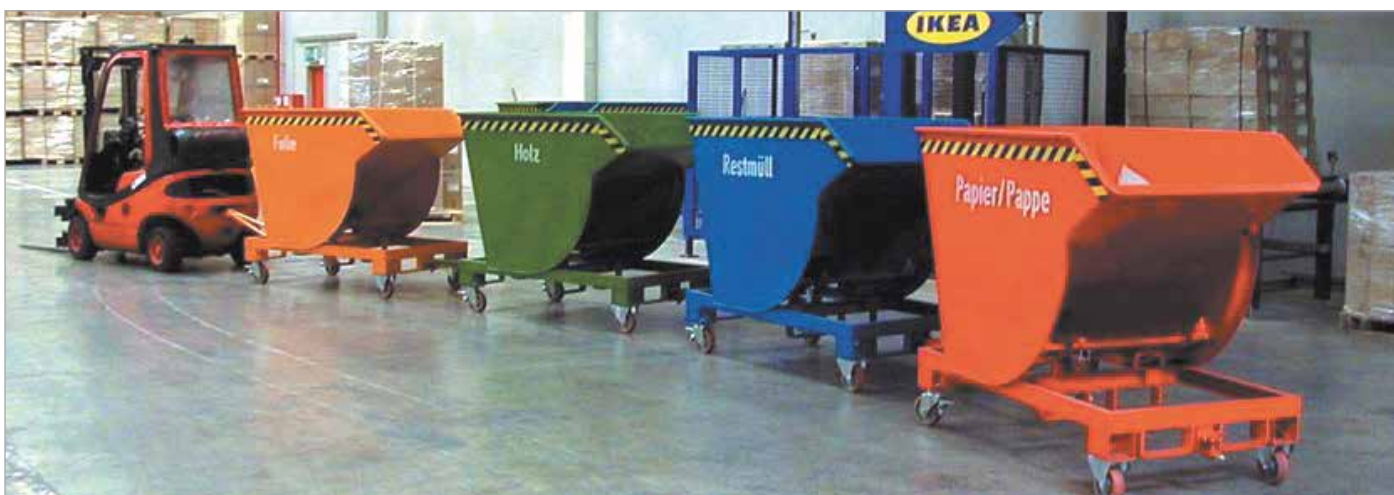
BKM with castors, trailer coupling and towing bar
