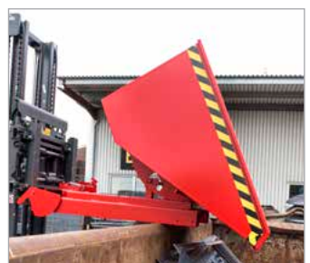
Emptied by activating release point 2
