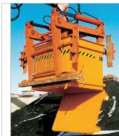
BC with brick clamp operated trap door
