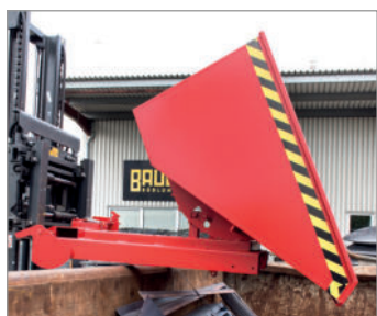
Emptied by activating release point 3
