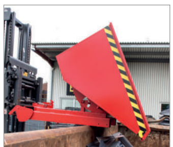
Emptied by activating release point 2
