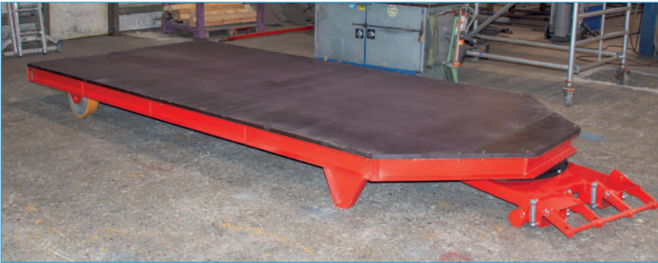
STS with anti-slip "Betosieb" boards
