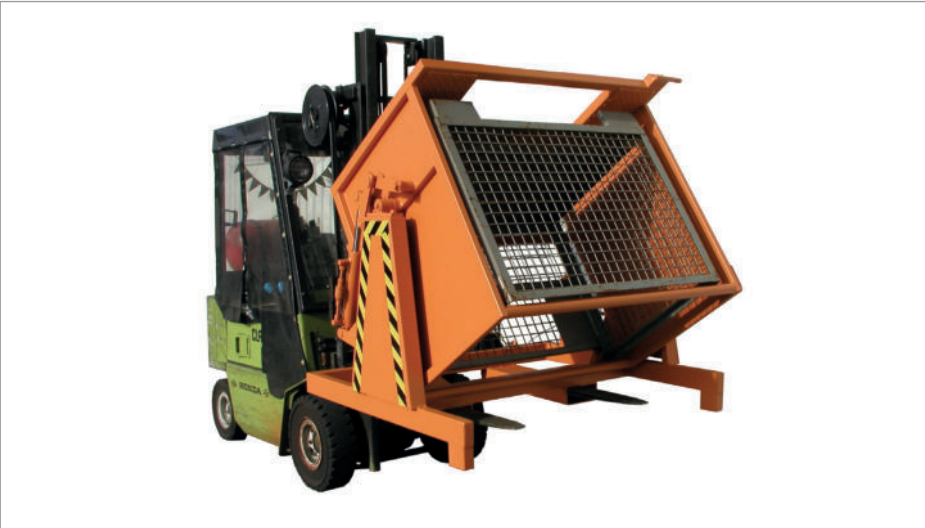
KGM with adjustable dumping brake
