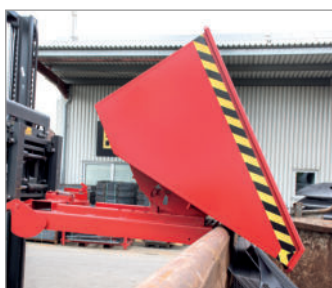
Emptied by activating release point 1
